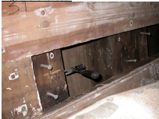
Fig. 3+4. Details of the construction of the hull: Rafters approx. 26*26cm covered on both sides with planks of approx 8cm thickness. Distance of rafters approx. 40cm.
