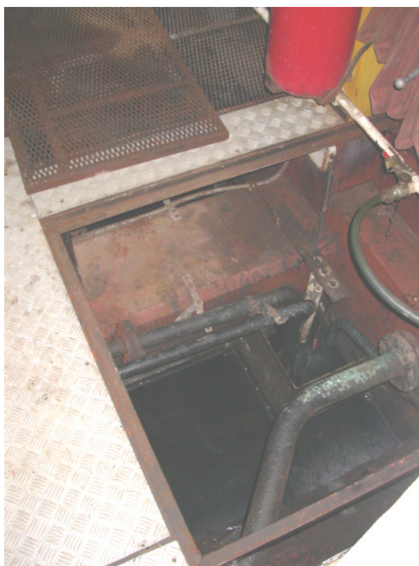
Fig. 10: Bilge below the technical room: Water is continuously standing at the keel which is normal for any vessel. No signs of decay were found.
