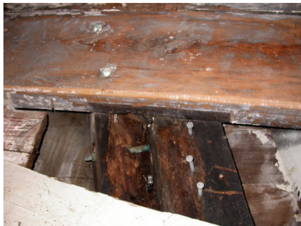
Fig. 3+4. Details of the construction of the hull: Rafters approx. 26*26cm covered on both sides with planks of approx 8cm thickness. Distance of rafters approx. 40cm.
