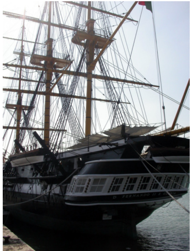
Fig. 12: the highly structured rear part gives many water traps.
