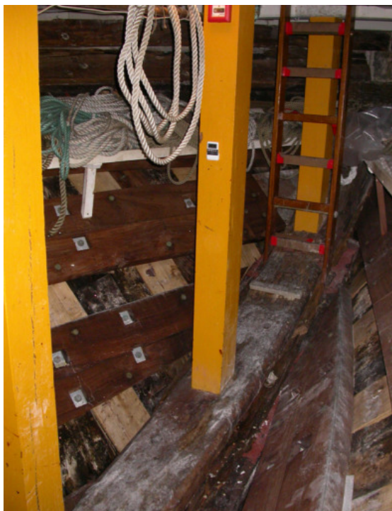
Fig. 7: (left) Bow-room. Traces of floating water are visible but know the wood is at acceptable equilibrium moisture. Some deteriorated rafters are replaced by laminated and on site glued wood that is unfortunately of Spruce ( Picea ssp. ) with no natural durability (!).
